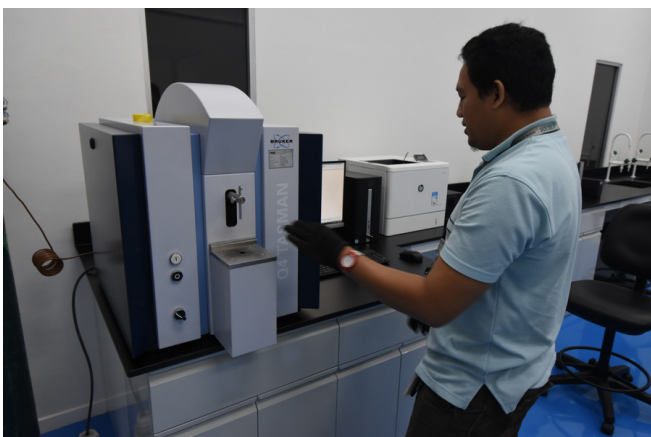
Spectrometer to determine chemical composition of iron & steel
