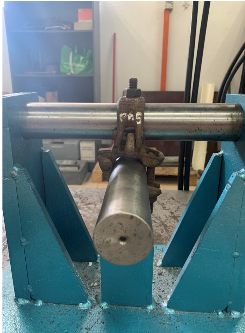
Load test on coupler
