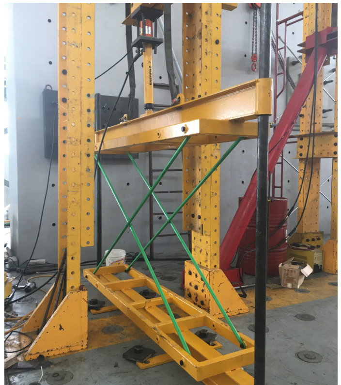
Load test of cross brace
