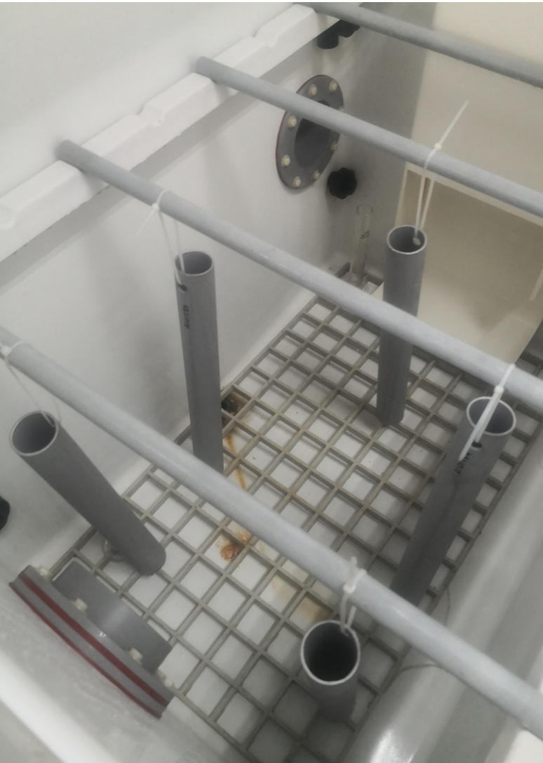
Corrosion test on scaffolding tube
