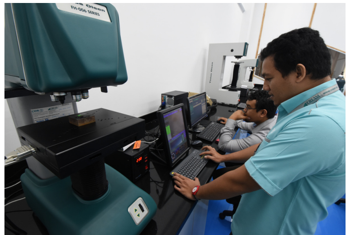
Hardness testing machine to determine hardness properties of iron & steel
