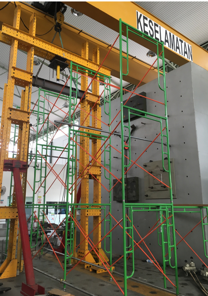
Full scale test on A-Frame scaffolding
