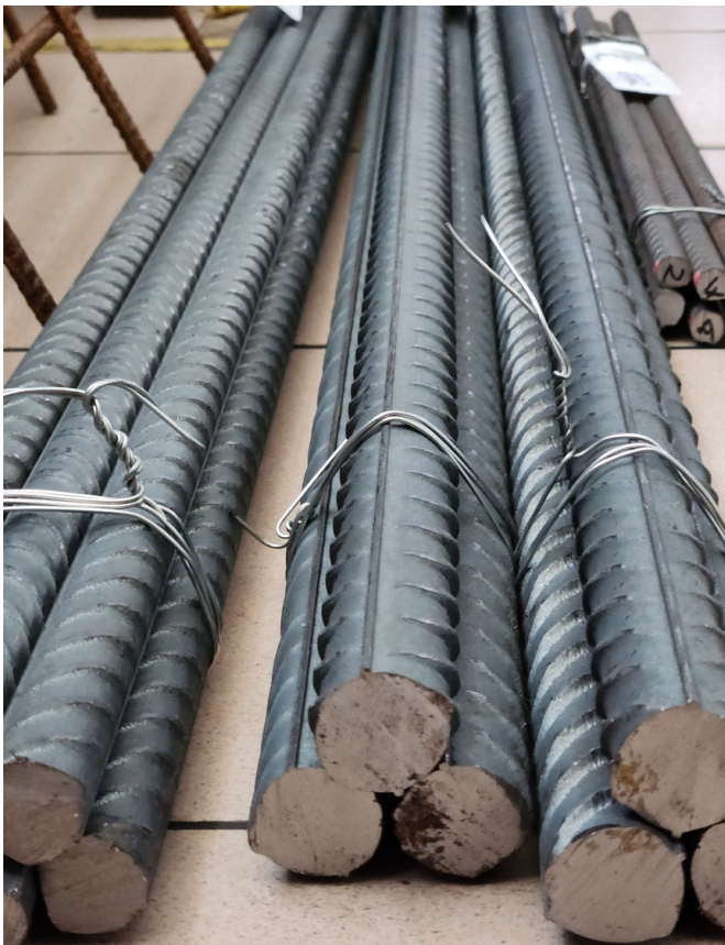
Hot rolled steel reinforcement bar (rebar)
