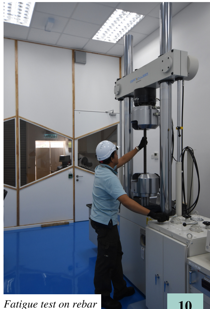
Typical tensile test using 2000 kN capacity UTM
